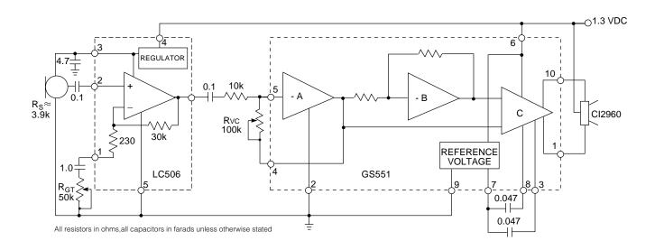
Fig. 3 Application Circuit
